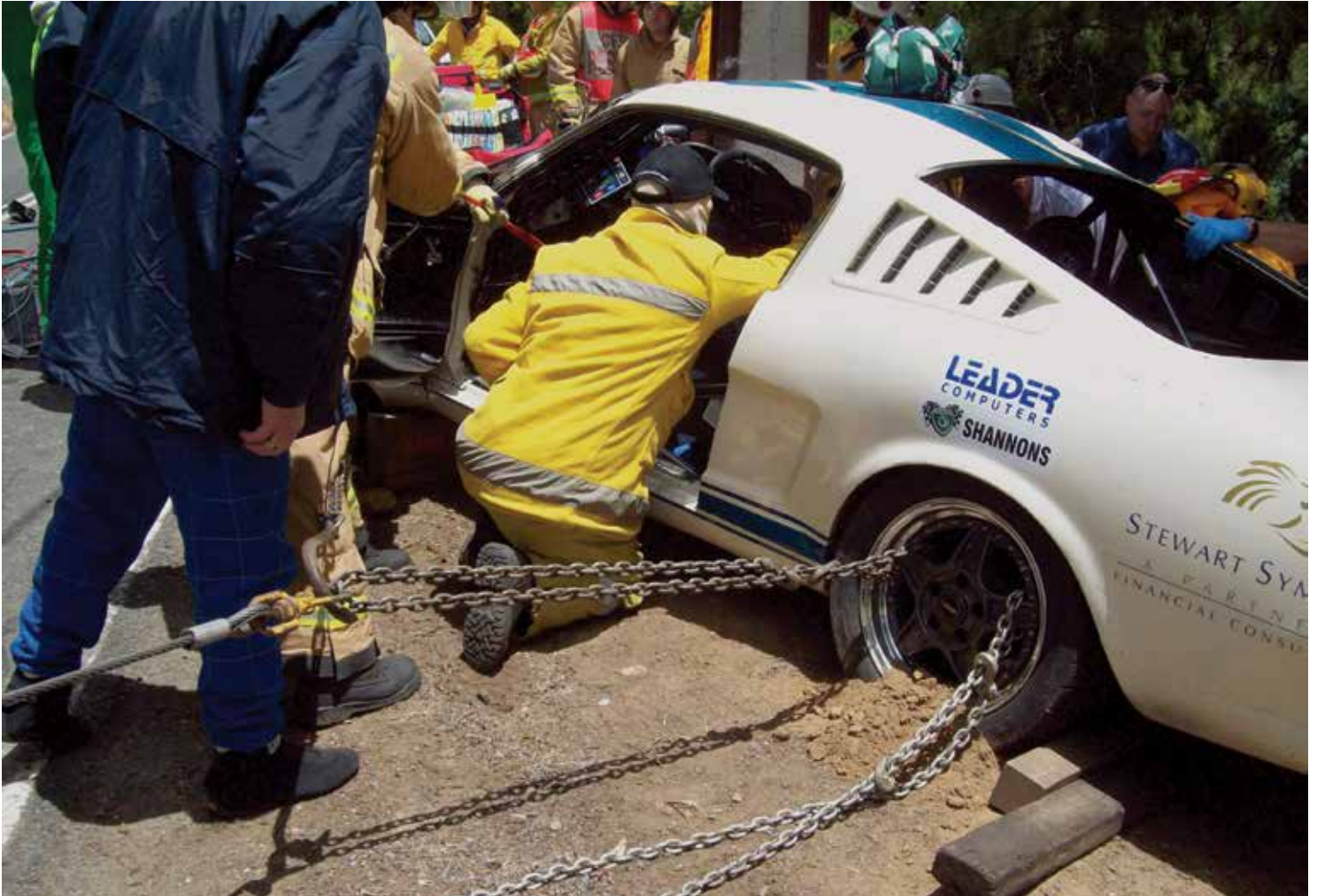
Moving crashed vehicles is an under used technique that speeds up extrication
