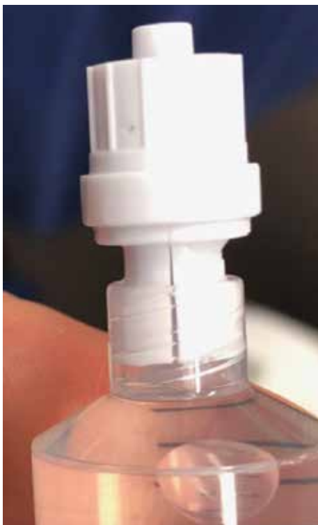
A cracked anti-reflux valve.
